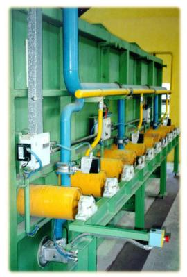
The unit is designed to pre-heat and dry material to be treated such as drying before sandblasting operations and sufficient pre-heating before painting operations.
